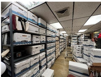
File boxes stored too close to ceiling
