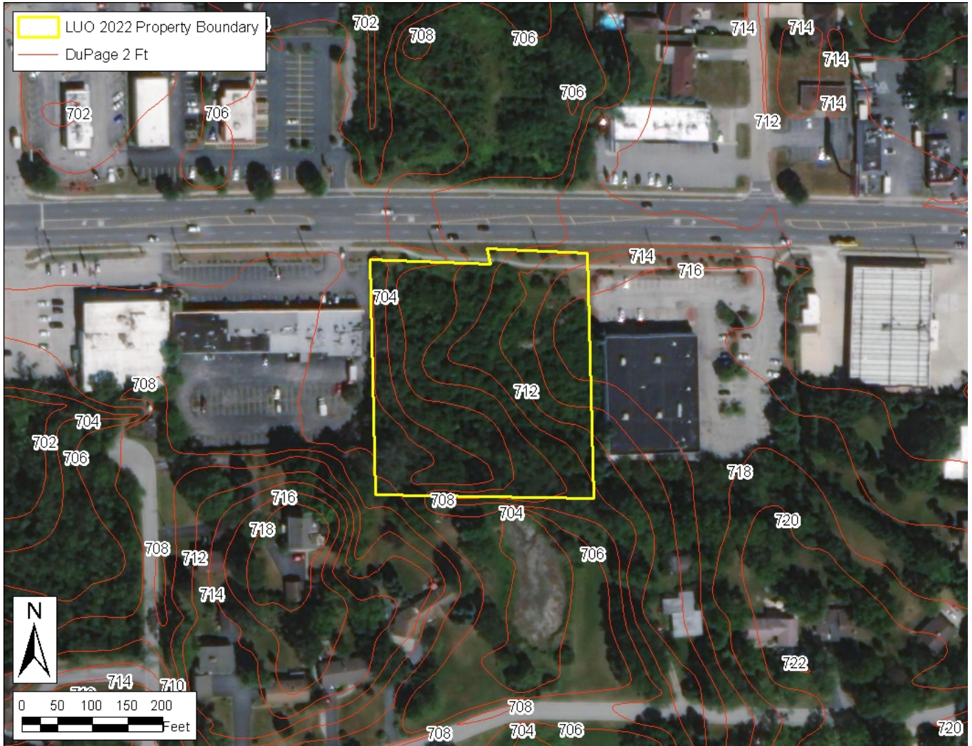
Figure 7: Topographic map showing contour lines
