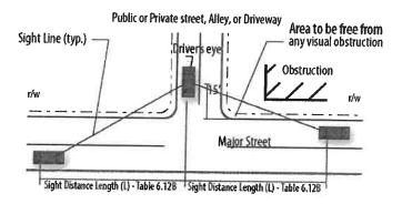
Figure 28-3E in the IDOT Bureau of Local Roads & Streets (BLRS) presents the sight distance requirements for a minor road, that is 2-way stop controlled:
