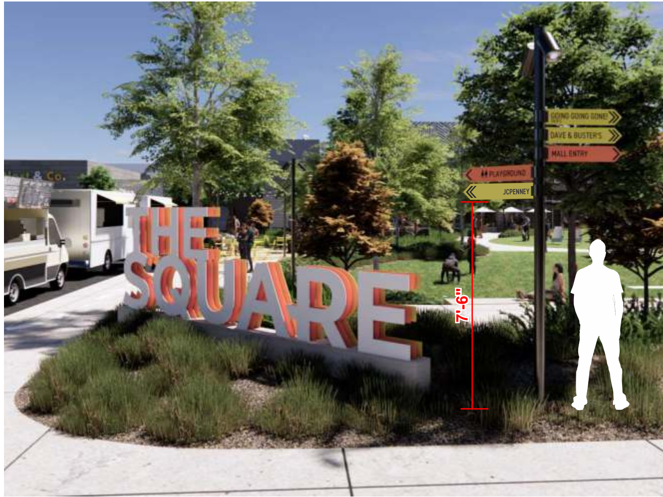
Minimum Height from Grade to Lowest Panel : 7'-6"
