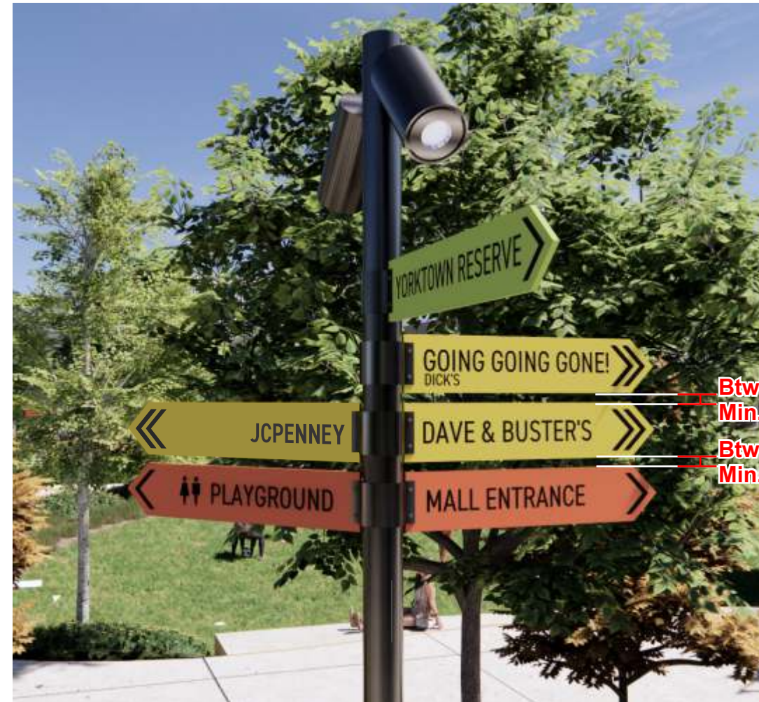
Max. 6 Destinations per Post Min. 1" Spacing Between Arrows Provide single- and double-panel bracket systems. Double-panel brackets to include both 180° and 135° configurations. Refer to renderings for intended orientation. Submit final bracket design for approval prior to fabrication.
