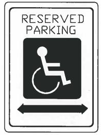
THIS IS A STANDARD SIGN AND MAY BE DRDERD FROM ANY TRAFFIC SIGN SUPPLIER BY NUMBER. THE ARROW SHOULD BE DNLY DNE SPACE. THE ARROW MAY ALSO BE MADE TO POINT IN DNLY DNE DIRECTION. THE SIGN MUST BE SUPPLEMENTED WITH THE ILLINDIS STANDARD R7-1101 PLATE GIVING THE AMOUNT OF THE FINE FOR ILLEGALLY PARKING IN THE RESERVED SPACE(S).
